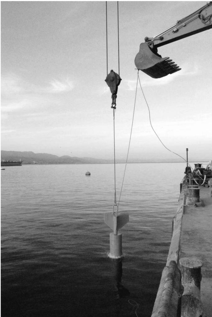
Figure 5. Start Corer's deployment
