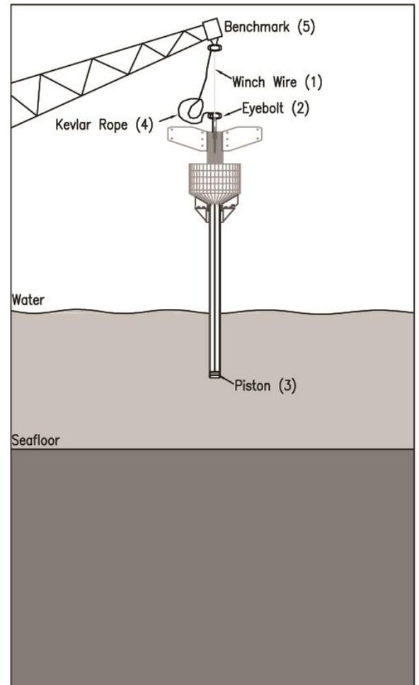
Figure 1. Set-up of Corer
