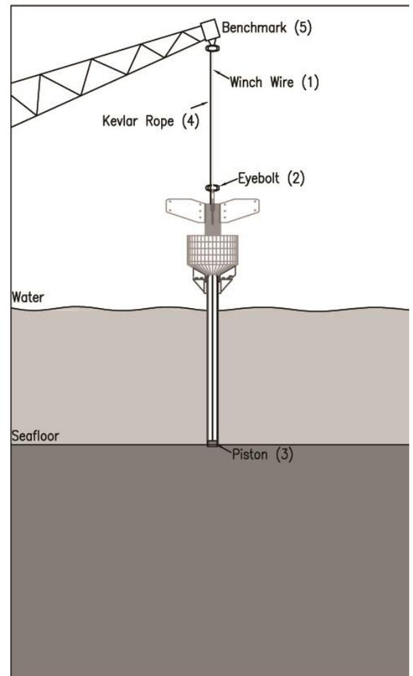
Figure 2. Initial coring phase
